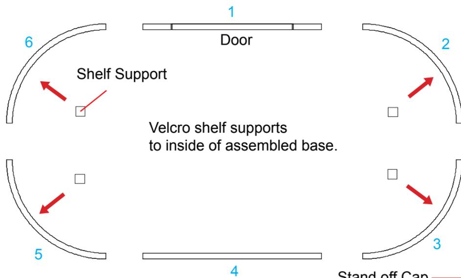
Insert stand off cap thru panel into connector located on the verticals as shown.
